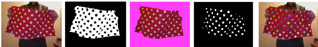
Figure 3: Polka dot detector. Left to right: original image, primary color mask, dot mask, augmented image
